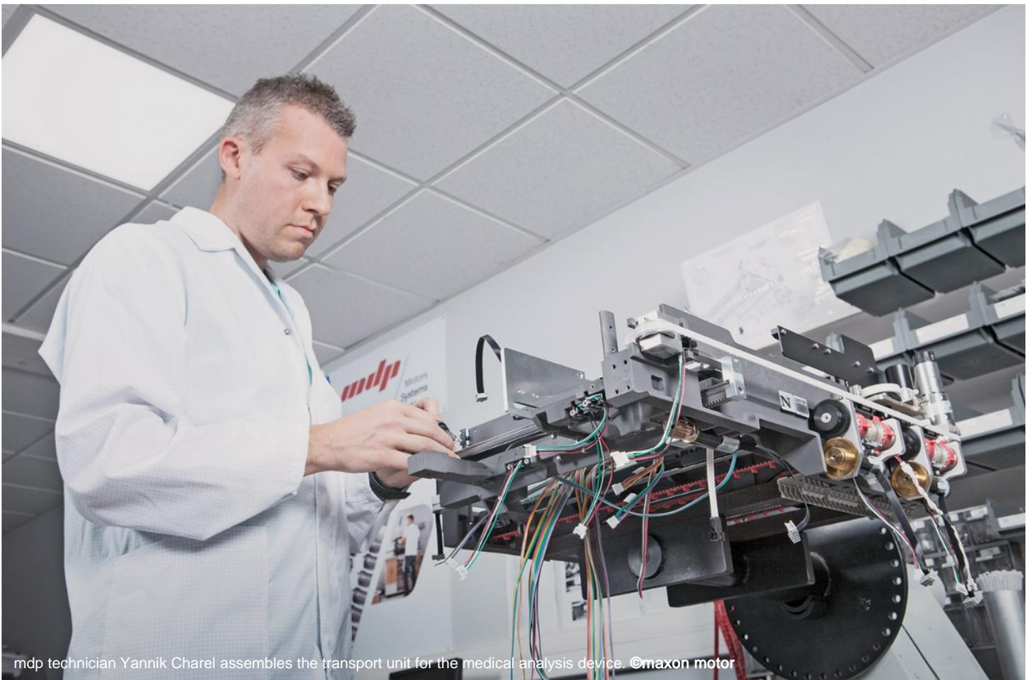
mdp technician Yannik Charel assembles the transport unit for the medical analysis device. ©maxon motor
